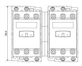
Dimension for 2 Pole contactor is same as dimension for 3 Pole contactor.
