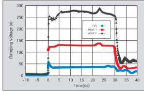
TVS Diodes have a significantly lower clamping voltage than the MOVs
