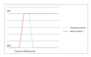
Timing diagram for de-latching and main contacts operation (For illustration purpose only)
