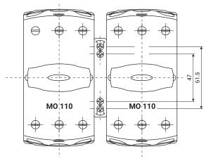
Note: Mechanical interlock kit can be fitted even with side auxiliary contacts in that case width will increase by 12 mm per auxiliary contact block.
