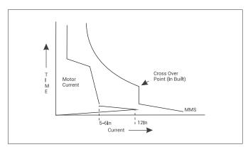
Hence, to avoid nuisance tripping, it is technically correct to increase the MMS rating for star/delta starting so that the ratio of instantaneous release setting to the motor full load current is at least 18. However, this will lead to loss in thermal overload protection offered by the MMS (as the MMS rating will be higher than the full load current of the motor). This aspect can be addressed by providing an additional thermal overload relay in the phase circuit.
