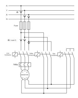
Starting current in a normal delta motor with DOL starting is around 6-8 times the motor full load current. However in Star-Delta starter motor starting current in star is reduced to 1/3rd of this value. Typically starting current when using Star-Delta starting method is around 2.2 times motor full load current.
