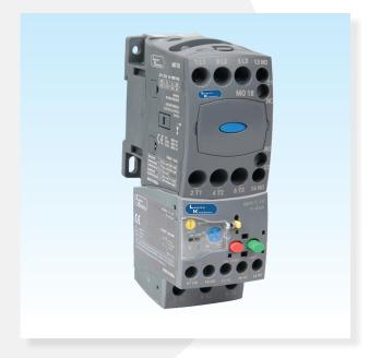
REO range of Electronic Overcurrent Relays to complete the portfolio of motor protection relays. These relays complement MO range of contactors as they have similar aesthetics as MO range and can be directly mounted on the same. The relays trip based on definite time characteristics. That is, the relay has settable Start time and Trip time.
