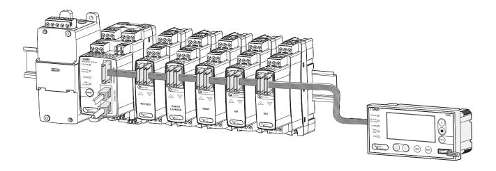
Note: Expansion module to be mounted on Right side of Main Unit.
