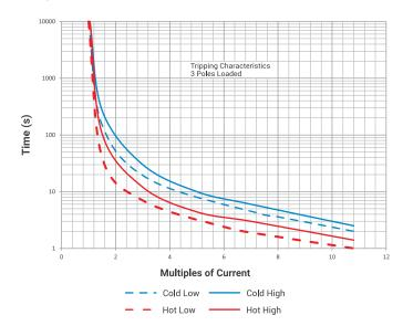
RTO-1 Relay On MO Frame O Contactor (9/12/18A)
