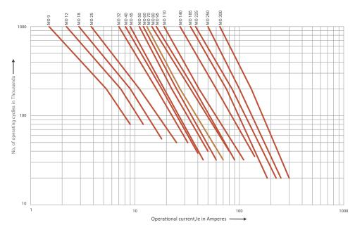
The Electrical life of MO 32 at 32A AC-4 is 50000. When a 32A contactor is used for 32AAC-4 application, one gets an operation life of 50000 operating cycles. If the contactor does approximately 500 switching cycles per week then the contactor will last for a period of 50000/500 = 100 weeks i.e. roughly 2 years.
